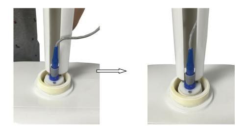
Attention: Remaining cable needs to be secured inside the notch. Failure to secure the cable may cause damage resulting in malfunction of height measurement.
